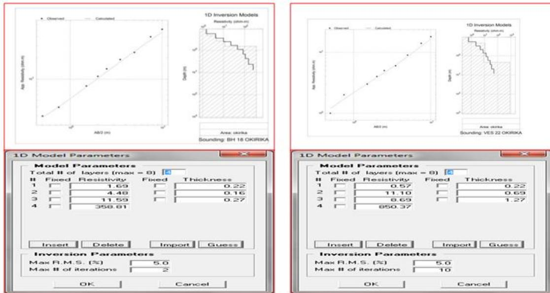
Fig 2b: Typical VES curve obtained at the contaminated site (Okirika).
