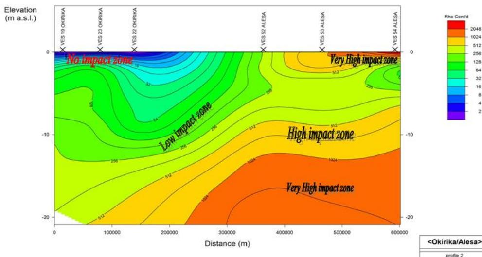
Fig. 3 (a and b): Geoelectric section of the study areas showing the level of contamination
